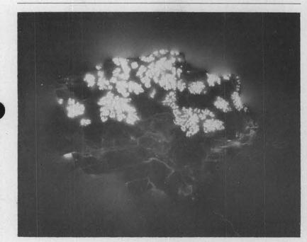
RADIATION AT WORK-Pegmatite ore placed on a loaded film holder produced this spectacular exposure after 40 hours. The bright spots are from pitchblend radiation and the dimmer lines were made by uraninite. See the accompanying story.
